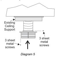
The connection between the appliance and the Retro Connector may be completed with sections of black direct vent pipe, together with an adjustable length.
